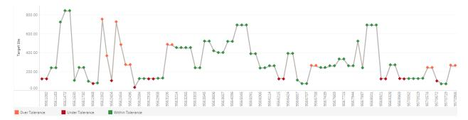
The manager of the feed mill recognized this data was relevant regarding the performance of the frequency drive on the liquid pump. He proceeded to make an adjustment by reducing the full speed and the freefall speed settings the pump had been operating at. This allowed the freefall weights of Fat AV Blend to be more consistent and resulted in a vast improvement in accuracy (as illustrated in the following chart) produced after implementing the process change:
