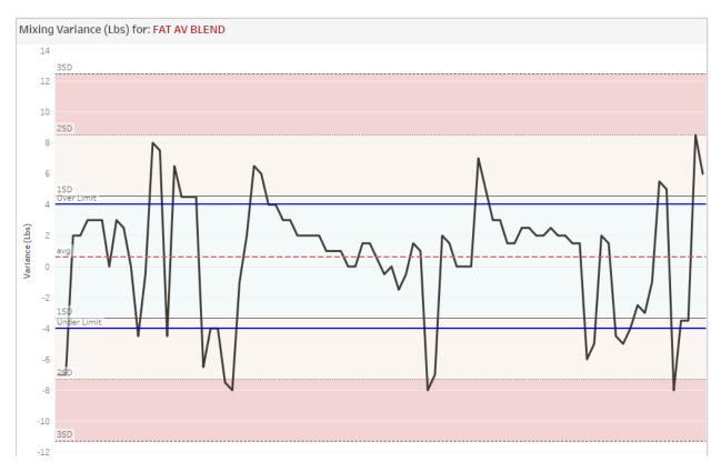
Note the blue lines on the chart indicating the tight Over/Under limits for Fat AV Blend at this mill, with the pounds of variation from each of the 90 batches containing this ingredient illustrated by the black line. The red dashed line represents the average variation over these 90 batches of 0.59 lbs. The light green, yellow, and red "channels" in the chart are drawn at the points of standard deviation (SD) as a statistical reference.
